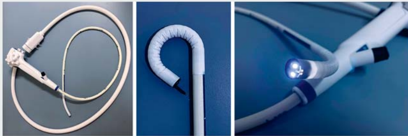
► Fig. 1 The Ambu aScope Gastro single-use device: diameter 9.9 mm; working channel 2.8 mm; bending angle, up 210°, down 90°, left 100°, right 100°; and equipped with two light-emitting diodes (LEDs).
